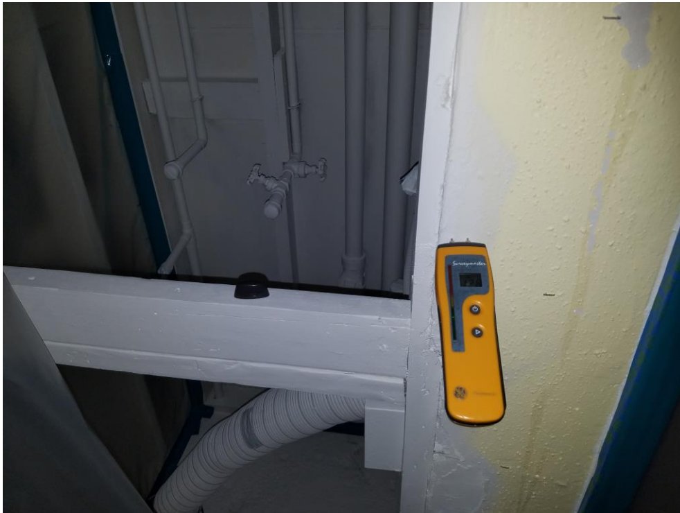
Hall sheetrock is dry, reading 12.9%
