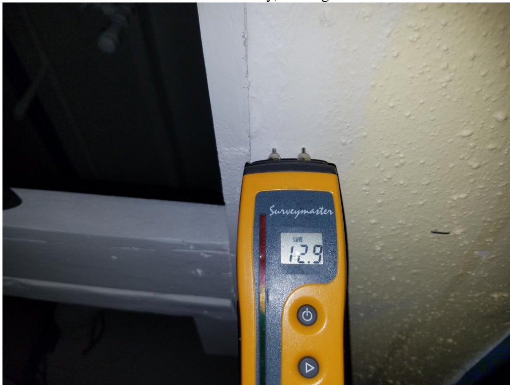
Hall sheetrock is dry, reading 12.9%
