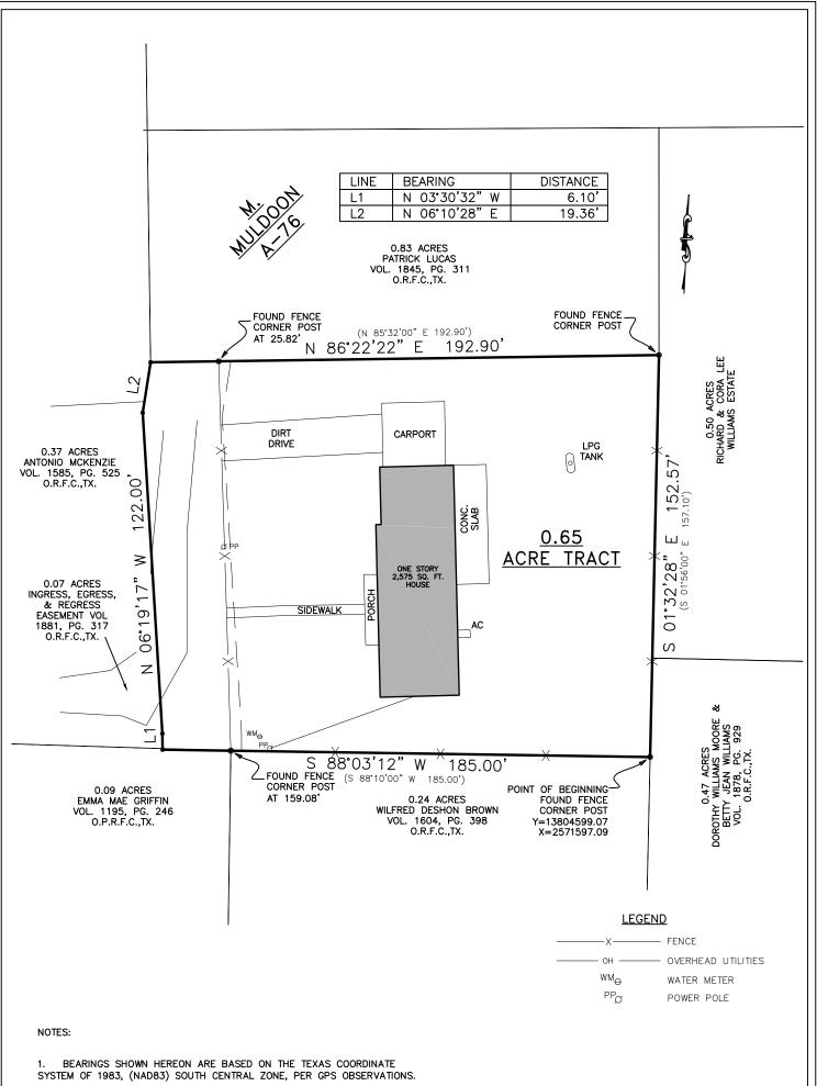
2. (BEARING DISTANCE) INDICATES RECORD BEARING AND DISTANCE.
