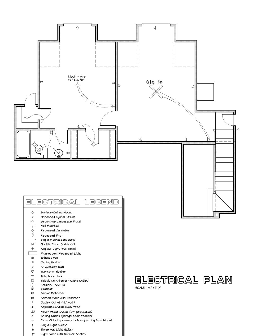
Ceiling Fan (provide proper ceiling brace)
