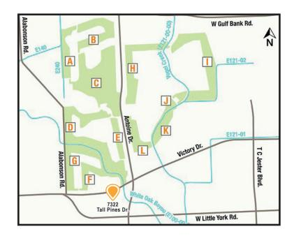
The City of Houston is currently working with the Flood Control District to finalize the design and begin construction of Phase One, which includes Basin E as well as portions of Basins C and D. The project expects to create an estimated 300 acre-feet of new storage with this phase. Construction is anticipated to begin in October.
