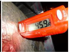
Note: A measure of how well an air conditioning system is operating is called "Delta T" and is the difference in temperature between the air going into the system and the air coming out. The acceptable range is 17 to 21 degrees.
