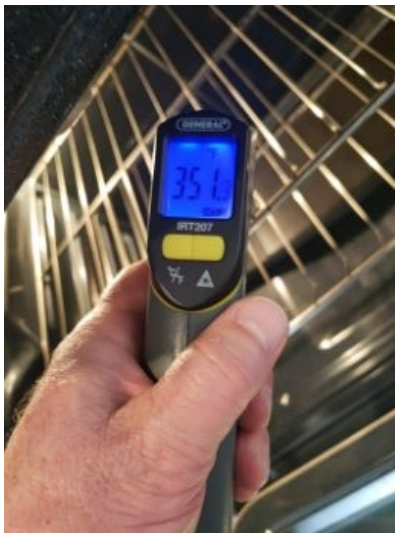
The oven was set on bake at 350 degrees and allowed to heat completely, and measured at 351 degrees (acceptable).
