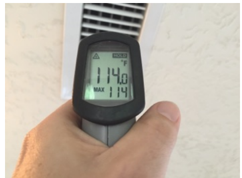
2nd floor hot air temperature
