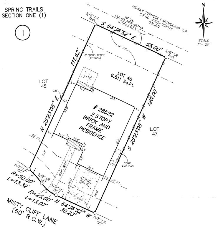
All bearings shown are based on the recorded plat referenced hereon.
