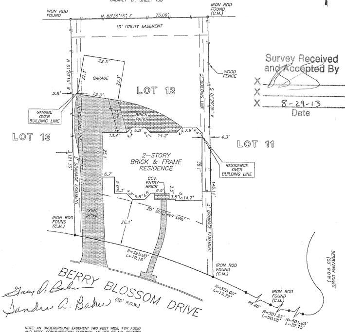
NOTE: AN UNDERGROUND EASEMENT TWO FEET WIDE, FOR AUDIO AND VIDEO COMMUNICATION FACILITIES, AS PER CF NO. 9026255.
