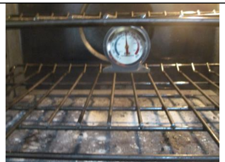
Oven temperature detected at 350°F. Oven operating as intended, within +/- 25°F of 350°F setting.
