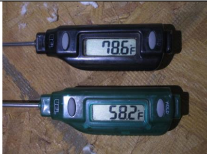
System temp. differential 20.6°F
