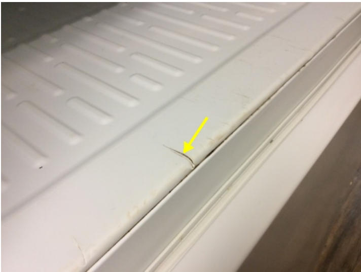
The gasket in the freezer compartment of the refrigerator is damaged and allows ice to form around the edge
