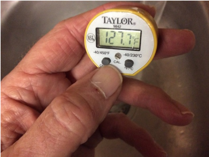
Hot water temperature measured at the kitchen sink 127.7°
