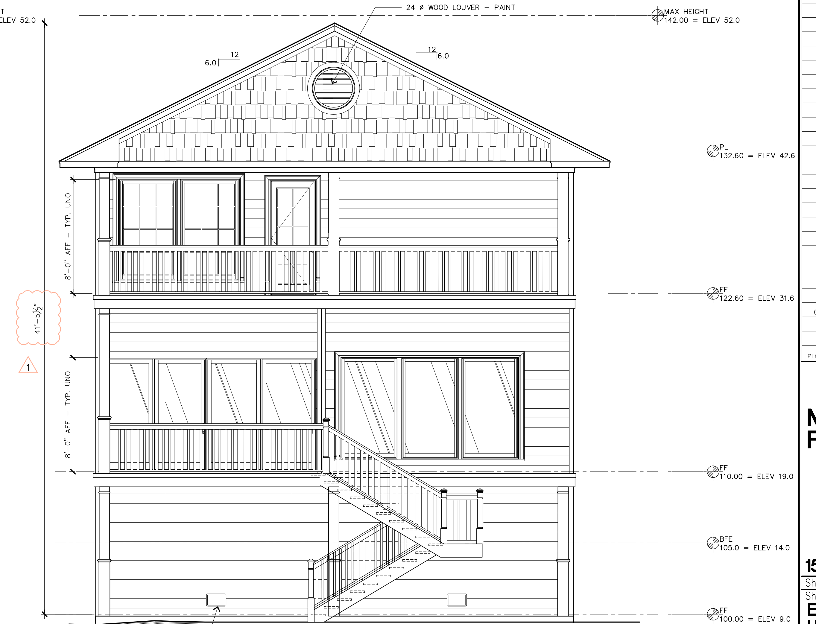
3 EXTERIOR ELEVATION NORTH WALL 1/4 = 1-0
