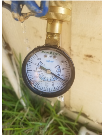
Static water pressure was observed to be: 50 psi. The acceptable range for residential water pressure is 40 to 80 psi.
