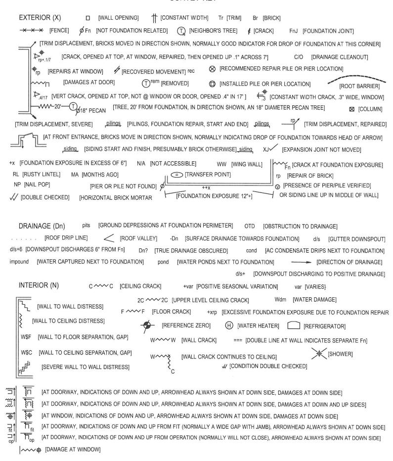
ALL DAMAGES NOTED ON SURVEY PRESUMED TO BE FROM FOUNDATION MOVEMENT MOST COMMON NOTATIONS SHOWN, LESS COMMON NOTATIONS DERIVED OR WRITTEN OUT
