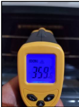
Oven set to 350, within acceptable range 359.6
