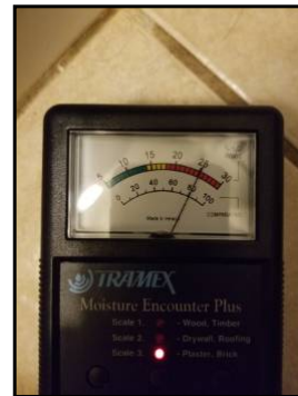
Hallway bathroom tub, 25%
