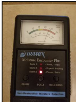
Hallway bathroom control, 23%
