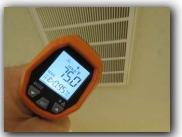
☑ Unit #2:downstairs Return Air Temp: 76 °F Temp. Differential: 13 °F Supply Air Temp: 63 °F
