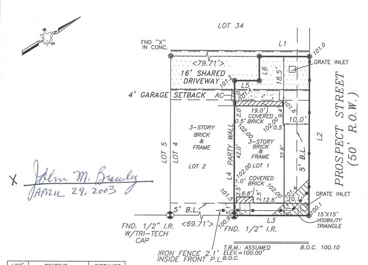
LINE BEARING DISTANCE L1 N 32°19'01" E 20.29 S 57°40'59" E 12 65.58' L3 S 32'19'01" W 30.29 L4 N 57°40'59" W 55.58 15 N 32°19'01" E 10.00 L6 N 57°40'59" W 10.00'
