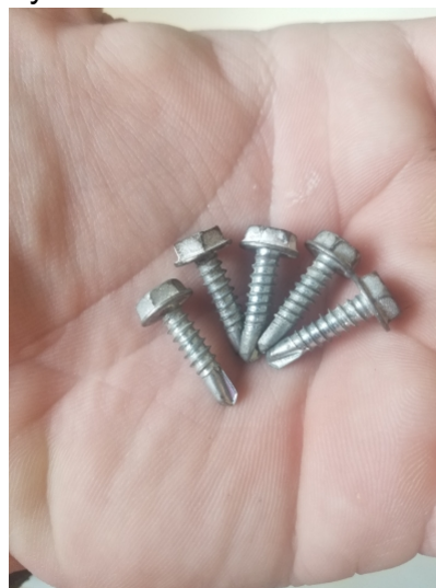
Pointed screw fasteners installed to secure metal "dead-front" cover on electrical panel box which is an "electrical-hazard" and screws can penetrate wiring inside box (replace with blunted-end type screws).
