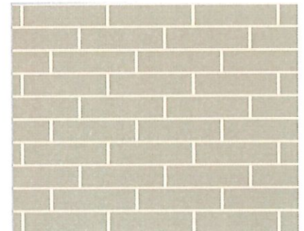
Tile Layout option 2 Staggered 33% horizontally (upgrade)
