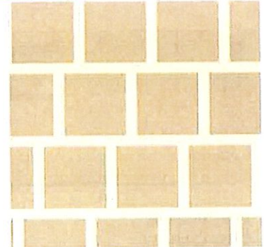
Tile Layout option 2 Flooring laid 33% offset Upgrade
