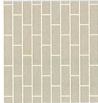
Tile Layout option 2 Flooring laid 33% offset Upgrade
