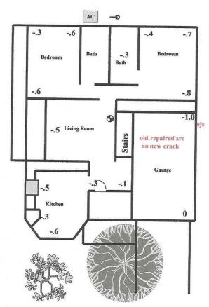
The home is within engineering tolerance limits, and appears to be stable with minimal stress. Recommend resealing expansion joint with new epoxy.
