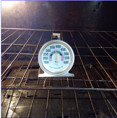
D. Item 5(Picture) Oven tested at 350° (within the 25° differential)
