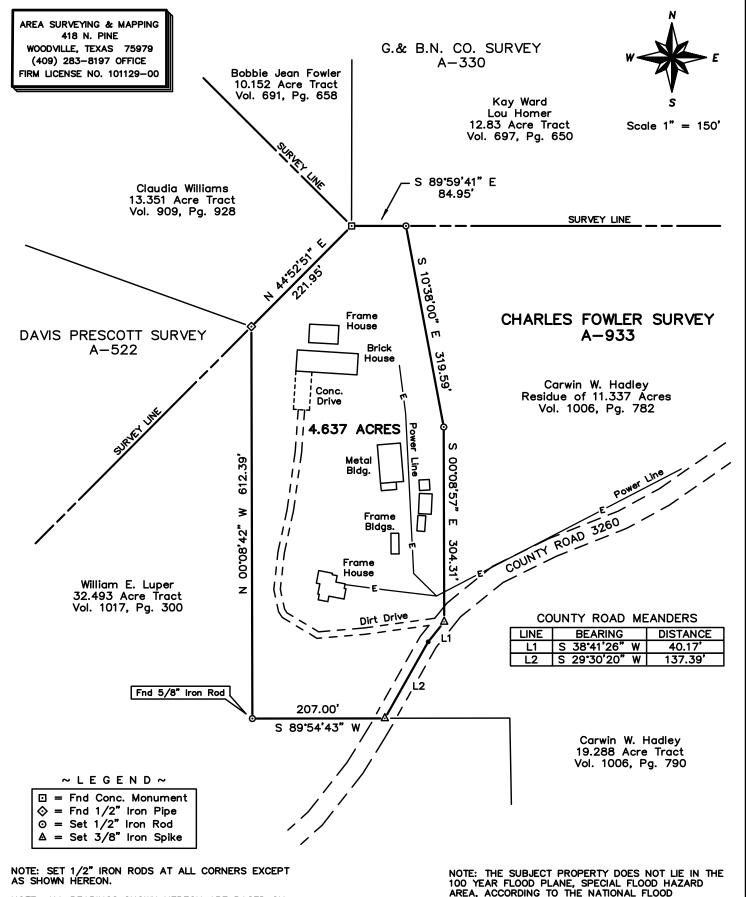
NOTE: ALL BEARINGS SHOWN HEREON ARE BASED ON AND/OR ROTATED TO THE NORTH LINE OF THE CARWIN W. HADLEY 11.337 ACRE TRACT. (S 89'59'41" E)
