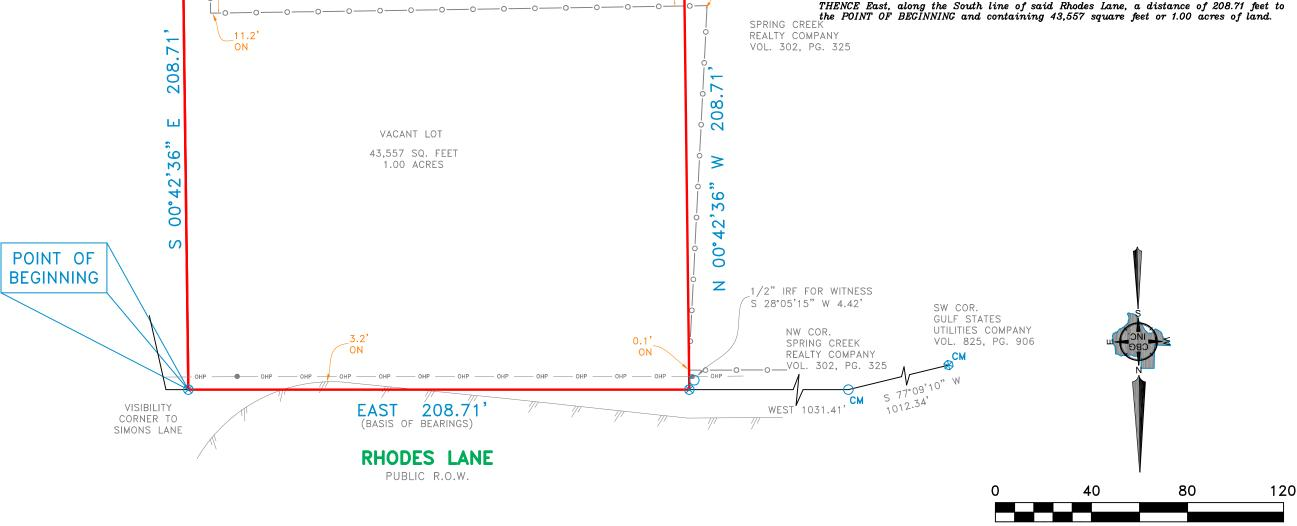
BEARINGS ARE BASED ON DEED RECORDED IN VOL. 302, PG. 325. EASEMENTS AND BUILDING LINES ARE BY RECORDED PLAT UNLESS OTHERWISE NOTED.
