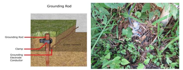
> The installed grounding clamp at the ground rod is for use in a natural gas pipe application. Grounding rods are required to have an acorn grounding clamp.
