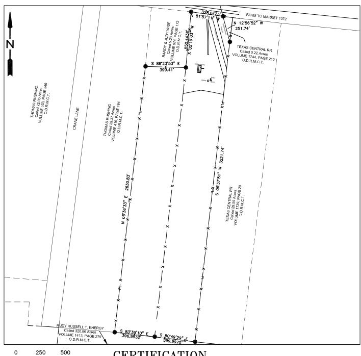
Basis of Bearings for this Survey is **Grid North from GPS Observation TEXAS S. CENTRAL 4204 NAD83**
