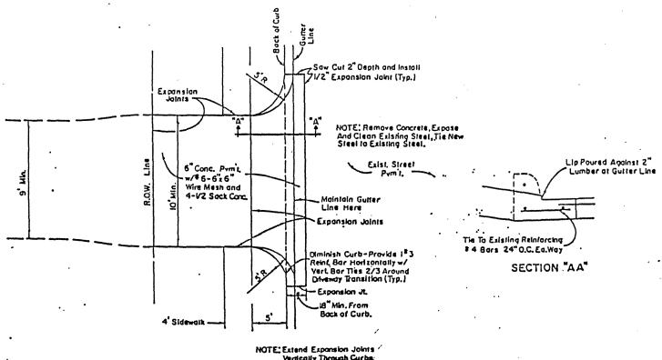
NOTE: Extend Expansion Joints Vertically Through Curbs:
