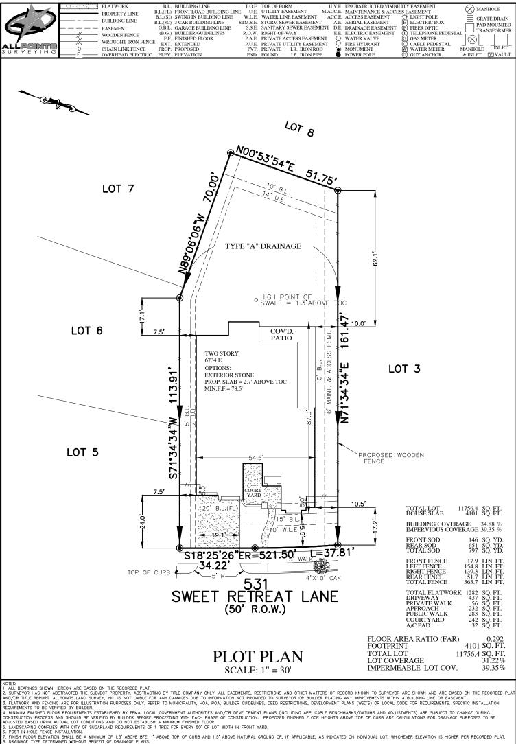
FLOOR ELEVATION SHALL BE A MINIMUM OF 1.5' ABOVE BFE, 1' ABOVE TOP OF CURB AND 1.5' ABOVE NATURAL GROUND OR, IF APPLICABLE, AS INDICATED ON INDIVIDUAL LOT, WHICHEVER ELEVATION IS HIGHER PER RECORDED PLAT. OR TOP OF THE DETERMINED WITHOUT BENEFIT OF DRAINAGE PLANS.
