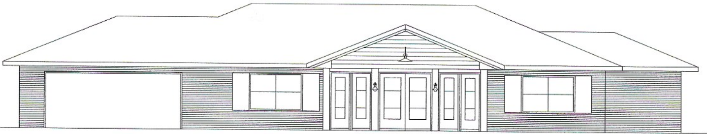
NEW WOOD + GLASS ENTRY ADDITION GABLE ROOF
