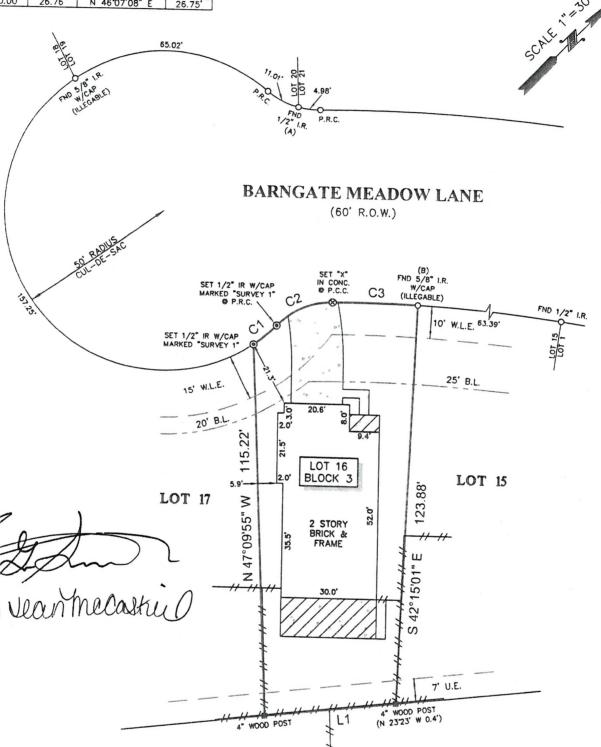
ALL BEARINGS SHOWN HEREON ARE REFERENCED TO THE SUBDIVISION PLAT NAMED BELOW, POINTS (A) AND (B) WERE HELD FOR HORIZONTAL CONTROL.
