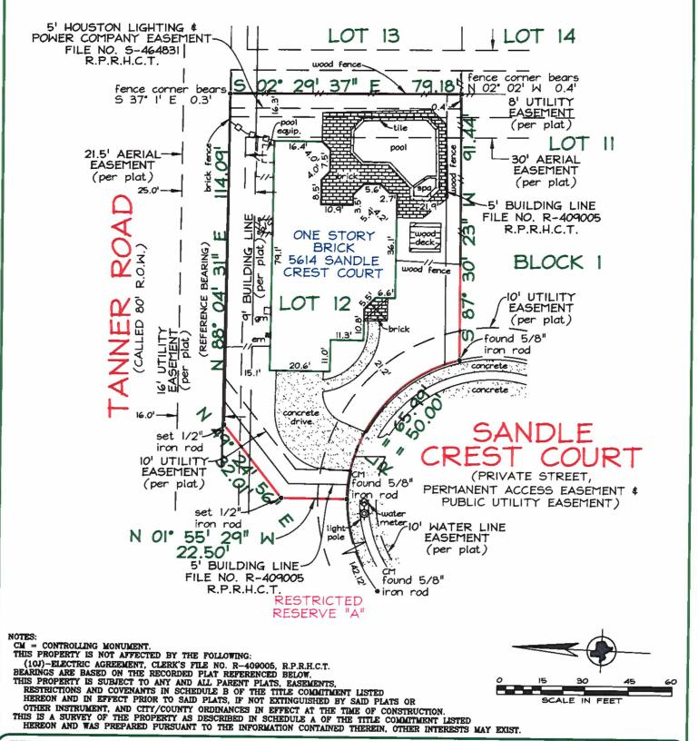
THIS IS TO DECLARE that on this date a survey was made on the ground, under my direction and supervision of the property located at 5614 SANDLE CREST COURT, and Being Lot Twelve (12), in Block One (1), of LAKES ON ELDRIDGE, SECTION ELEVEN (11), REPLAT, an addition in Harris County, Texas, according to the map or plat thereof recorded in Film Code No. 381077 of the Map Records of Harris County, Texas.
