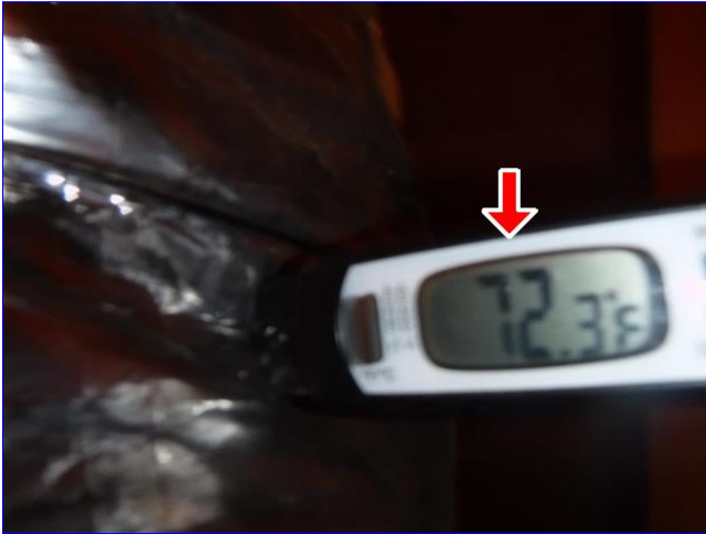
B. Item 1(Picture) View of the cooling system measured return air temperature at the evaporator.
