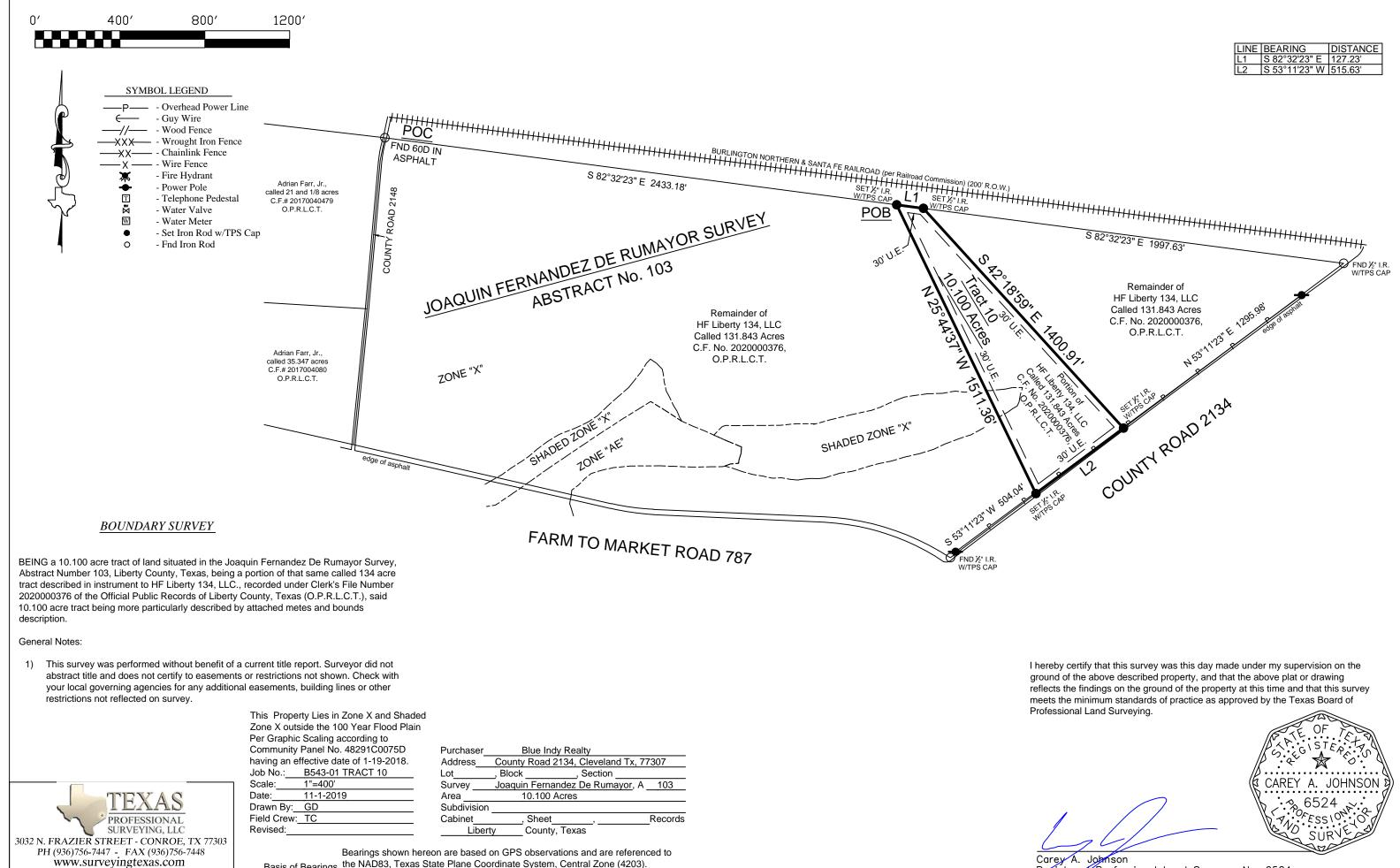
Basis of Bearings the NAD83, Texas State Plane Coordinate System, Central Zone (4203).
