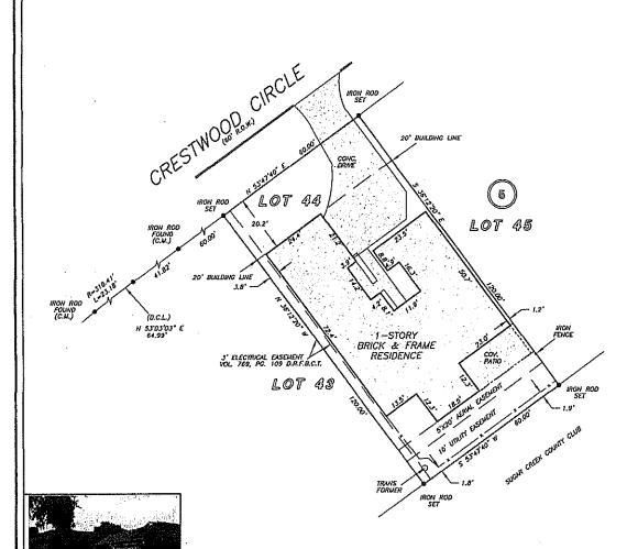
HOTE: ENTEX INC. EASEMENT AS PER VOL. 769, PG. 109. NOTE: FORT BEND CO. DRAIN EASEMENT AS PER VOL. 774, PG. 864 & VOL. 809, PG. 887.
