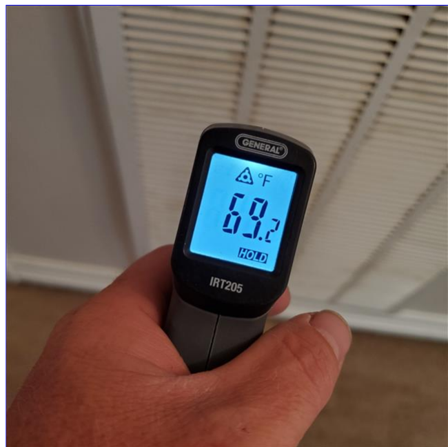
B. Item 1(Picture) The return air temperature was approximately 69 degrees. There should be a 14 to 22 degree drop between return and Supply air temperature.
