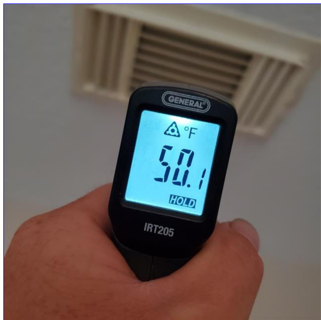
B. Item 2(Picture) Supply air temperature was approximately 50 degrees. There was a 19 degree drop between return and supply air temperature, indicating the cooling equipment was cooling adequately at time of inspection.
