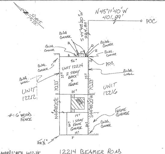
A=S4511'40"E L=17.3B' B=N4448'20"E L=3.00" C=S4511'40"E L=6.00" D=S4448'20"W L=3.00 E=S4511'40"E L=2.57 F=N4511'40"W L=26.00'
