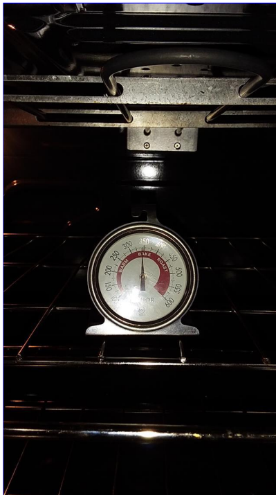
D. Item 4(Picture) lower oven tested at 350 degrees
