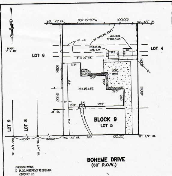
2) METAL BLDG. ON BRICK FLOOR ONTO 10' I.E.
