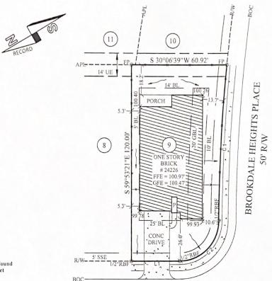
LEGEND: RBF- Rebar Found RBS- Rebar Set P-Porch BL- Building Line GBL-Garage Building Line WLE- Water Line Easement **UE-** Utility Easement R/W- Right of Way APL- Approximate Property Line BOC- Back of Curb FFE- Finished Floor Elevation GFE- Garage Floor Elevation CONC- Concrete -X- Fence FP- Fence Post
