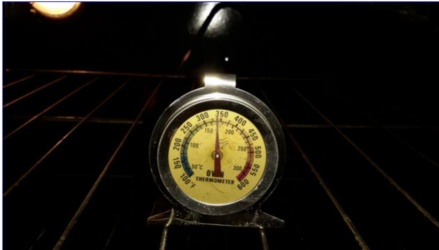
D. Item 2(Picture) oven tested at 350 degrees
