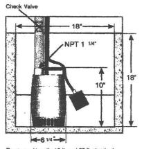
Power cord length: 10 ft. and 25 ft. standard, float switch length: 10ft. and 25ft. available. 18" sump size recommended for best operation of wide angle mercury float switch.
