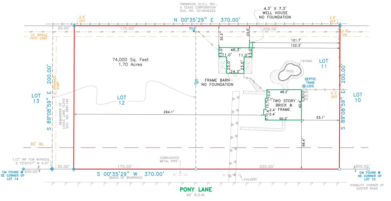
BEARINGS, EASEMENTS AND BUILDING LINES ARE BY RECORDED PLAT UNLESS FLOOD NOTE: According to the F.I.R.M. No. 48157C0080L, this property does lie in Zone AE and DOES lie within the 100 year flood zone.
