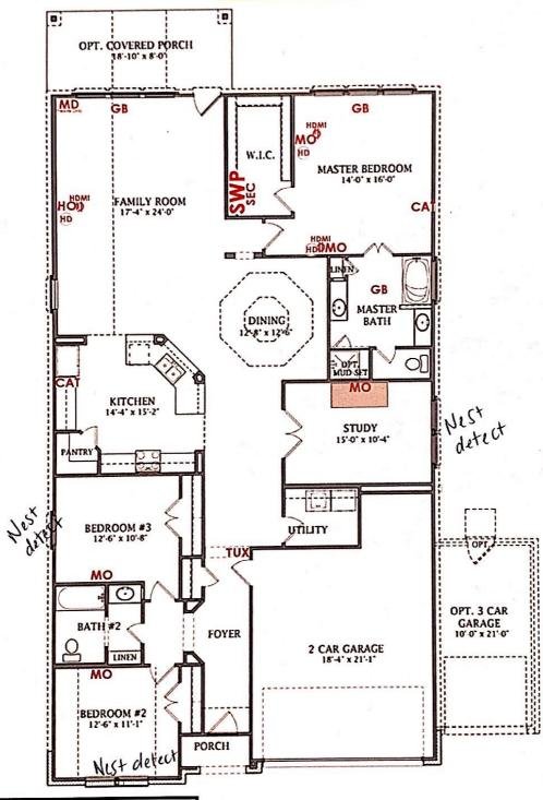
All markings are PREWIRED ONLY, FINISHED OUT/INSTALLED EQUIPMENT locations will be marked with inverted markings. EXAMPLES: CAM SP SP
