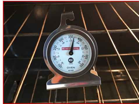
Oven set to 350 degrees, after 20 min oven is within specs, it would still benefit from adjustment
