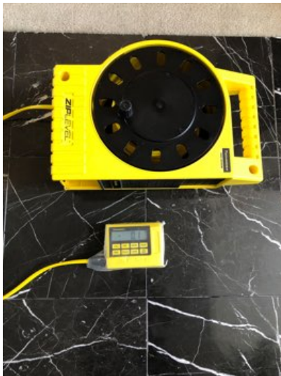
The foundation was inspected with a digital level. No deficiencies were found.
