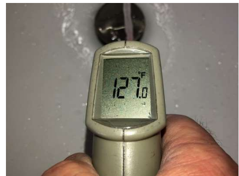
2nd floor: Hot water temperature: Scalding
