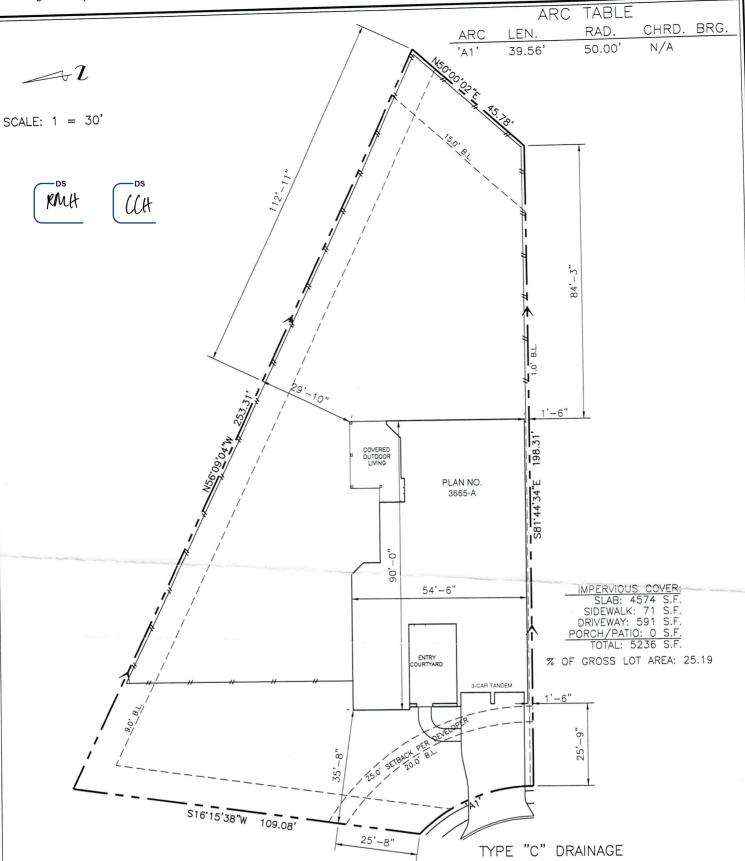
Note: This plot plan has been prepared without the use of a grading plan. The house pad elevation and site grades need to be field verified/established. The builder shall maintain 2% slope 5' away from the pad and  $1\ 1/2\%$  along side property lines.
