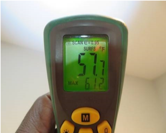
Average temperature reading from all supply registers.
