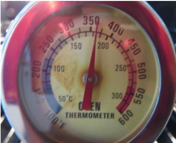
Oven set to 350 degrees and measured at 365 degrees - Unit should be re-calibrated.
