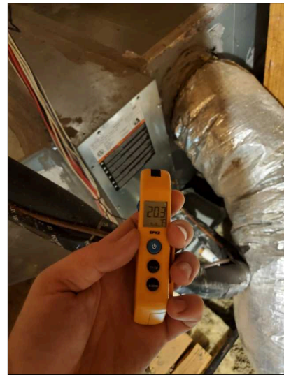
20f delta T across coil is acceptable. Downstairs
