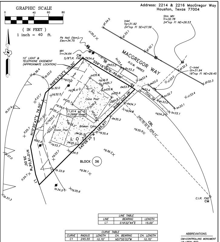
ELEVATIONS ARE REFERENCED TO RM 040090, BEING A BRASS DISK STAMPED D100 BM12 WITH AN ELEVATION OF 41.08 NAVDB8, 2001 ADJUSTMENT
