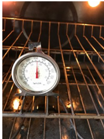
Whirlpool electric oven was measured at 345-355 degrees when set at 350 degrees.
